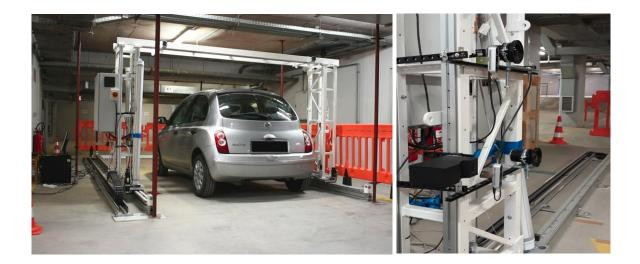
The scanning frame includes several cameras on each side to scan the car parked underneath. The operator enters the license plate of the inspected vehicle before starting the scanning process. When the 3D color model is ready the user can inspect the acquired images and, as an additional feature, manually annotate different types of defects on each image.
